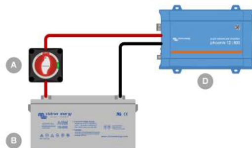
Battery Switch used to disconnect an inverter from the house battery. Use to preserve battery charge, system maintenance or in an emergency.
