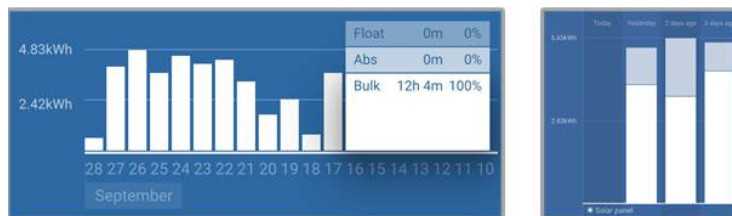
System spending all its time in bulk with breakdown of charge stages - System in bulk and absorption
